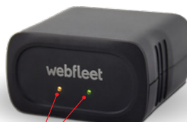
2 x LEDs for system and connection status
